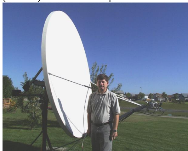
Figure 1 2.4 m Offset Reflector for 24/47 GHz
